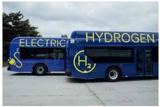
Advancement of our "side by side" pilot test of two zero emissions buses will inform the technology the agency uses to power its buses in the future. The agency's first battery electric bus (BEB) and hydrogen fuel cell electric bus (FCEB) will transport customers throughout our service area, while mechanics and planners gather data on how those technologies work relative to each other and to traditional diesel-powered buses.
